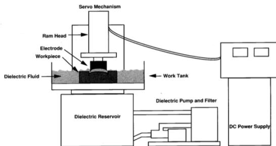
Figure – 1.1 Line Diagram of Basic EDM System
