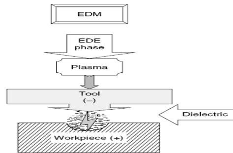
Figure –1.2 Working principal of EDM .
